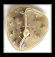
HEART SCULPTED IN PLASTILINE AND MOULDED IN FIBREGLASS IN 3 PARTS. THE FASTCAST CORE PIECE IS ONLY USED IF TRYING TO CREATE A HOLLOWED OUT HEART IN SILICONE RUBBER
