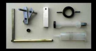
THE BALLOONS INSIDE THE HEART ARE CONTROLLED BY AIR-FILLED SYRINGES POWERED BY A CRANK MECHANISM TURNED BY HAND. CONSTRUCTED OUT OF TAPPED SILVER STEEL RODS, TURNED NYLON, MILD STEEL AND ALUMINIUM
